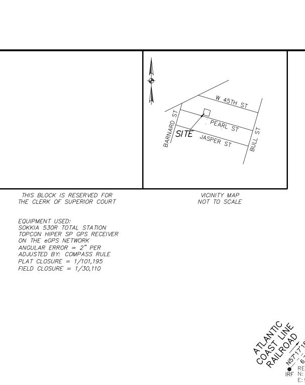
SURVEYOR'S NOTES 1. ALL COORDINATES AND BEARINGS ARE BASED ON GEORGIA STATE PLANE COORDINATE SYSTEM, NAD 83, EAST ZONE.
