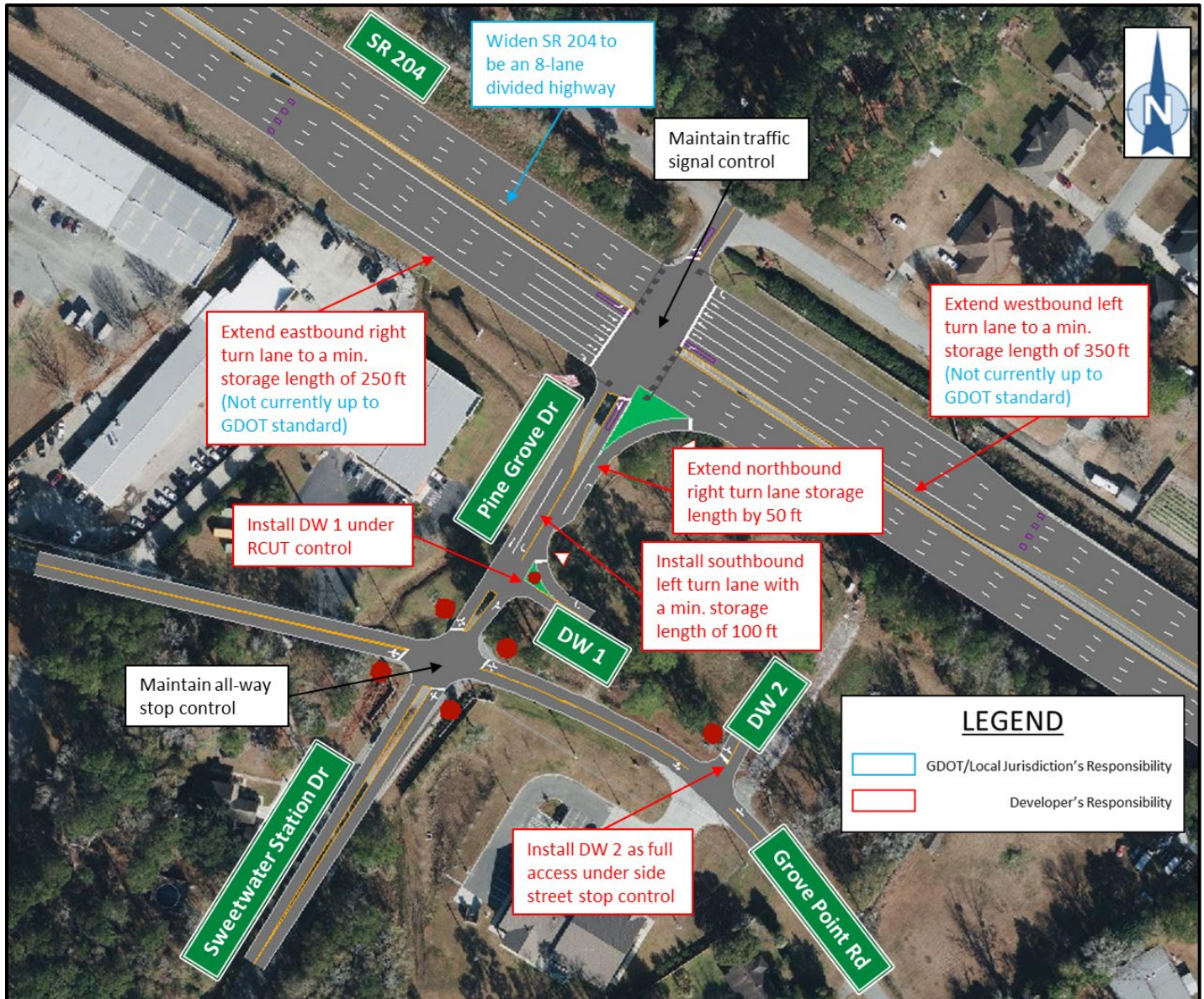
Figure 19: RECOMMENDATIONS – DW 1 AS RCUT
