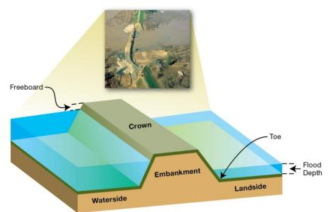
Figure 5.11 – Components of a Typical Levee
