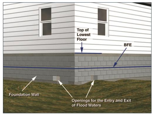
Figure C.1 – Building Codes and Flood Elevations
