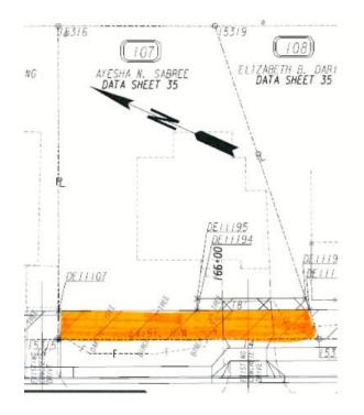
Orange shaded area indicates the proposed permanent easement for construction and maintenance of slopes.
