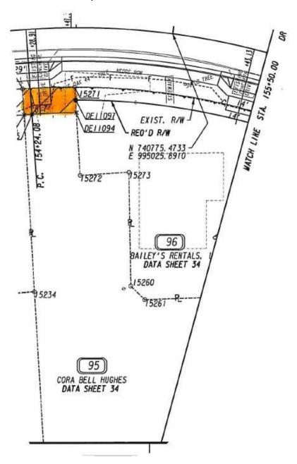
Orange shaded area indicates the proposed permanent easement for construction and maintenance of slopes.
