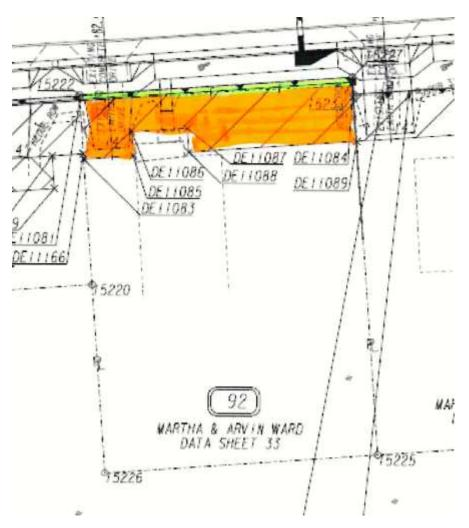
Orange shaded area indicates the proposed permanent easement for construction and maintenance of slopes.
