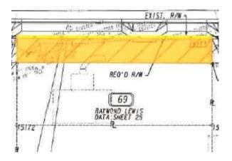
Orange shaded area indicates the proposed permanent easement for construction and maintenance of slopes.
