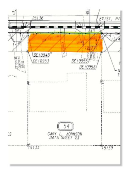
Orange shaded area indicates the proposed permanent easement for construction and maintenance of slopes.
