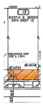
Orange shaded area indicates the proposed permanent easement for construction and maintenance of slopes.
