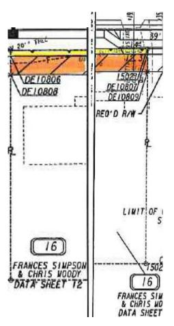
Orange shaded area indicates the proposed permanent easement for construction and maintenance of slopes.
