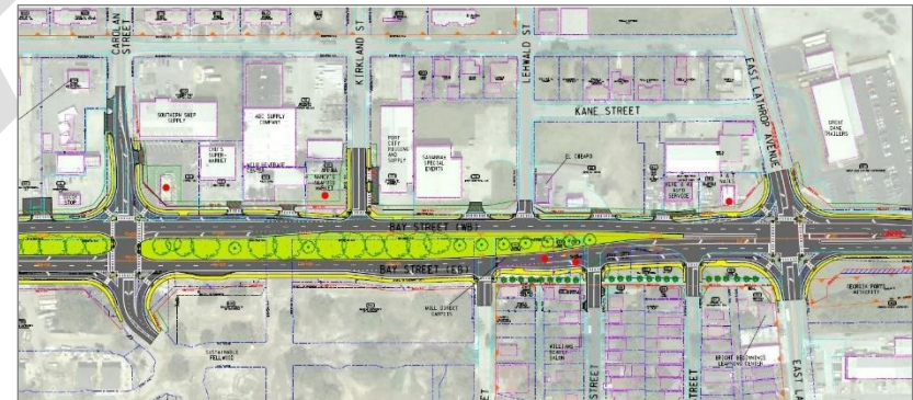
This section shows median, streetscape, and intersection improvements along West Bay Street between East Lathrop Avenue and Carolan Street. (Image: Georgia Department of Transportation)
