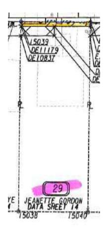
Orange shaded area indicates the proposed permanent easement for construction and maintenance of slopes.
