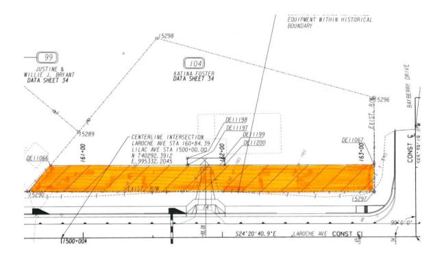
Orange shaded area indicates the proposed permanent easement for construction and maintenance of slopes.
