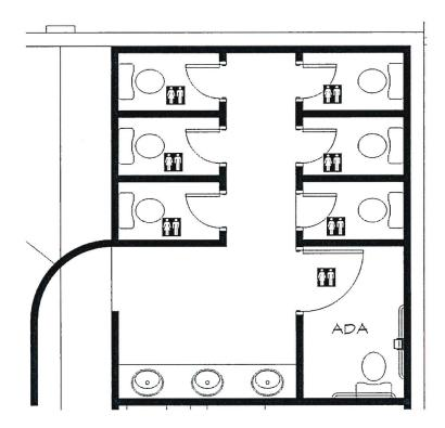
Bathroom example that meets the 2021 IPC. Water closets have walls from floor to ceiling but the sinks are located in the common area.
