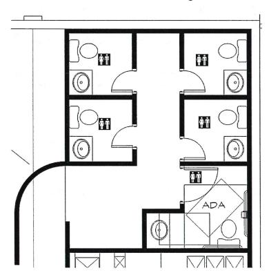
Bathroom example that meets current 2018 IPC. Water closets have walls from floor to ceiling and individual sinks.
