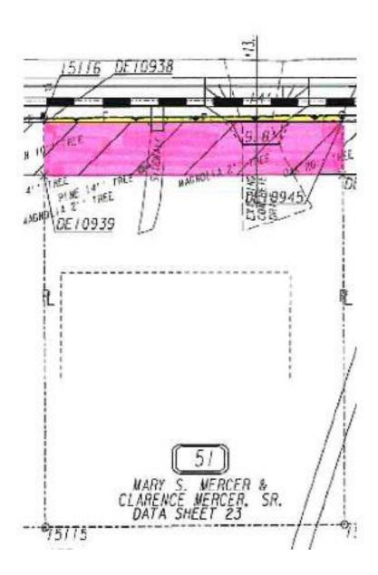
The area highlighted in pink indicates the proposed permanent easement for construction and maintenance of slopes.
